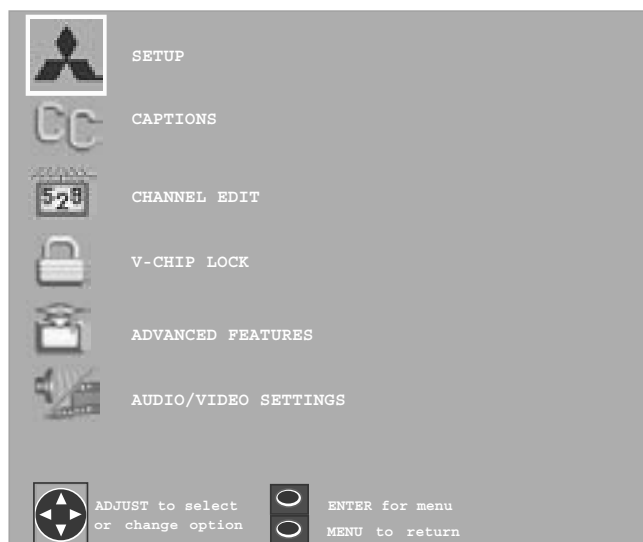
Figure 1. MAIN menu: The first screen to appear when you press MENU button on the remote.
